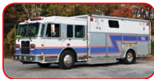
2004 EMI / Spartan Walk-In Rescue Cummins ISC 330 HP, Allison EVS3000 Onan 10KW PTO-Driven Generator 6-Bottle 6000psi Cascade System Hitch Receivers on Front and Rear Awning on Driver's Side
