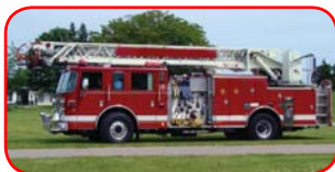
2004 Pierce Dash 75' Quint Caterpillar 455 HP Diesel Engine Allison EVS 4000P Automatic Hale QMAX 1500 GPM Pump 450 Gallon Poly Tank Monitor at Tip
