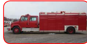
1994 Freightliner Heavy Rescue Cummins 8.3L 300 HP Diesel Engine Allison Automatic Transmission Winco 20KW PTO Generator Wilburt Light Tower
