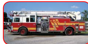
1996 Pierce Lance 75' Quint Detroit 8V92TA 500 HP Diesel Allison HD4060PR Automatic Hale QSMG150 1500 GPM Pump 300 Gallon Poly Tank Onan 6KW Diesel Generator
