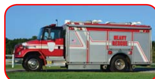
1997 Marion / FL Heavy Rescue Cat 3126 300 HP, Allison MD3060 PTO Driven Generator 2 - 4000W Telescoping Light Towers Air Compressor and Cascade System Awnings on Driver and Officer Sides
