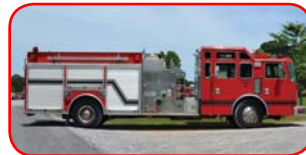
2002 KME Panther Rescue Pumper Detroit Series 50, Allison MD3060P Hale QMAX 1500 GPM Top-Mount Pump Foam Pro 2001 A & B System 750 Gallon Poly Tank 10Kw Hydraulic Generator
