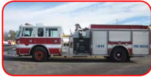
1994 Pierce Saber Rescue Pumper Detroit Diesel, Allison Automatic Waterous 1250 GPM Top-Mount Pump 750 Gallon Polypropylene Tank Akron Foam System 5KW Gas Generator
