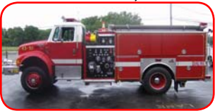
1998 Ferrara / Int'l 4x4 Pumper Int'l DT466E Diesel, Allison MT643 Hale QSG 1000 GPM Side-Mount Pump 750 Gallon Poly Tank Automatic Tire Chains, 12,000# Winch 4000 Watt Dynamote Inverter
