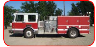
1992 Quality / Spartan Pumper Detroit 6V92TA, Allison HT740 Waterous 1250 GPM Side-Mount Pump 500 Gallon Fiberglass Tank Feecon ATP Foam System 50 Gallon Foam Tank
