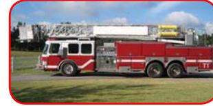
1991 E-One Hurricane 95' Platform Detroit 6V92TA 300 HP Diesel Allison MD3060 Automatic Hale QSMG 1250 GPM Pump 300 Gallon Poly Tank
