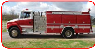
2000 Ferrara / Freightliner Pumper Cummins 8.3L 300 HP Diesel Engine Allison Automatic Transmission Hale QSG 1250 GPM Side-Mount Pump 1000 Gallon Poly Tank Feecon Foam System
