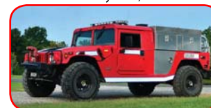
1997 AM General H-1 4x4 Brush Truck 6.5L Diesel Engine, Automatic Transmission Hale 250 GPM Pump 300 Gallon Poly Tank Sidewinder Remote Bumper Turret
