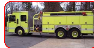
1999 Ferrara / Spartan Pumper Tanker Cummins 330 HP Diesel Allison Automatic Hale QSG 1250 GPM Top-Mount Pump 2000 Gallon Poly Tank Dump Valve in Rear
