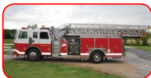
1991 Sutphen 75' Quint Detroit 8V92TA 445 HP Diesel Allison HT740D Automatic Hale QSMG 1500 GPM Pump 400 Gallon Fiberglass Tank
