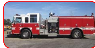
2001 Pierce Saber Rescue Pumper Cummins ISC 330 HP Diesel Allison MD3060 Automatic Waterous 1250 GPM Top-Mount Pump 750 Gallon Poly Tank FoamPro System w/ 20-Gallon Tank
