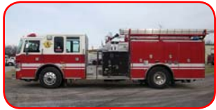
1997 Pierce Dash Rescue Pumper Detroit Series 40 Diesel Allison MD 3060 Automatic Waterous 1500 GPM Top-Mount Pump 500 Gallon Poly Tank
