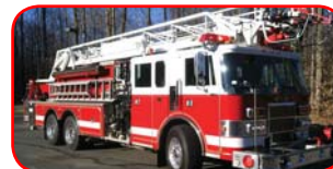
1992 Pierce Lance 75' Quint Detroit 8V92, Allison Automatic Waterous CMU 2000 GPM Pump 400 Gallon Poly Tank Waterway with Monitor at Tip Harrison 10KW Diesel Generator
