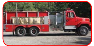
1983 4-Guys / Int'l Pumper Tanker Cummins 250 HP, Standard Transmission Hale 1000 GPM Side-Mount Pump 2250 Gallon Stainless Steel Tank Jet Dump on Rear
