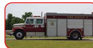
2001 Pierce / Int'l Heavy Rescue Int'l 330 HP, Allison MD3060 Onan 25KW PTO-Driven Generator 2 - Electric Reels, 1 - Hydraulic Reel 2 - Folding Light Towers Cascade System, Winch
