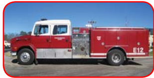
1997 Custom / Freightliner Pumper Detroit Series 55 Diesel Allison Automatic Transmission Waterous 1500 GPM Side-Mount Pump 500 Gallon Poly Tank
