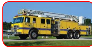
2002 Pierce Lance 75' Quint Cummins ISM 500 HP, Allison HD4060P Waterous CMU 2000 GPM Pump 00 Gallon Poly Tank AMPS 8KW Hydraulic Generator Interior Medical Cabinets
