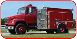
2001 Ferrara / Freightliner Pumper Cummins ISC 330 HP Diesel Allison MD3060 Automatic Darley 1000 GPM Side-Mount Pump 1000 Gallon Poly Tank
