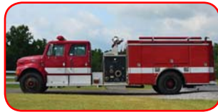
1999 Pierce / International Pumper Int'l 530 300 HP, Allison MD3060P Waterous 1250 GPM Top-Mount Pump 1000 Gallon Poly Tank 2 - Telescoping Scene Lights
