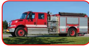
2007 Pierce / International Pumper Diesel Engine, Allison Automatic Hale 1250 GPM Side-Mount Pump 750 Gallon Poly Tank Foam Capable Pre-2010 Emissions
