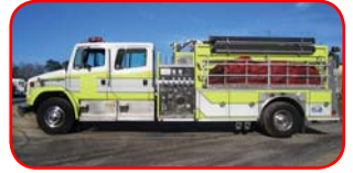
1998 E-One / FL Pumper / Tanker Cummins 325 HP Engine Allison HD Transmission Waterous 1250 GPM Pump 1800 Gallon Tank 2500 Gallon Portable Tank
