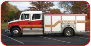
1999 Saulsbury / FL Rescue Pumper Detroit Series 50 Diesel Engine Allison Automatic Transmission Hale 1250 GPM Rear-Mount Pump 500 Gallon Poly Tank Deck Gun on Rear
